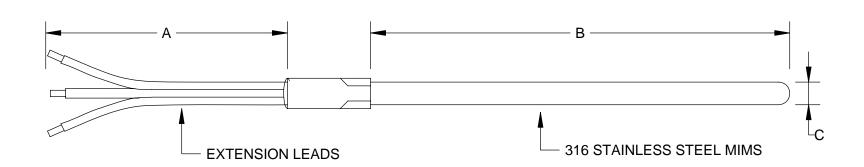
☐ CLASS B 3 WIRE SINGLE **4 WIRE SINGLE CLASS A** 6 WIRE DUPLEX 1\10 DIN
